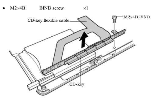
Figure 4-25 Removing the CD-key assembly
